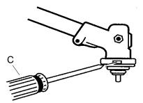
Screw on the trimmer head (D) in the opposite direction to the direction of rotation.
